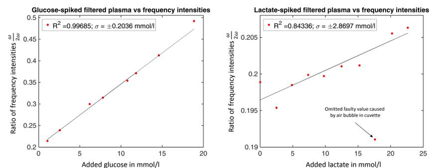
Fig. 4 – Correlation between concentration and intensity ratio of  $\omega$  and  $2\omega$  in protein-reduced spiked plasma samples. Left: glucose-spiked, right: lactate-spiked protein-reduced plasma. Faulty value caused by air bubble was omitted for  $R^2$  and  $\sigma$ -calculation.
