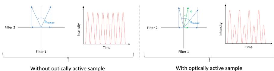
Fig. 2 – Principle of relation between optical rotation and detector intensity.
