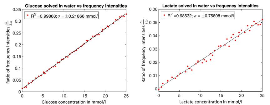
Fig. 3 – Correlation between concentration and intensity ratio of  $\omega$  and  $2\omega$  in water-solutions, left: D-glucose, right: sodium L-lactate.
