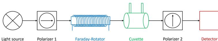
Fig. 1 – Polarizer measurement setup: Emitted light is polarized by polarizer 1 and modulated by Faraday-Rotator. Polarization is influenced by sample concentration, so that only rotated polarization can pass perpendicular polarizer 2. Signal is detected and further processed.
