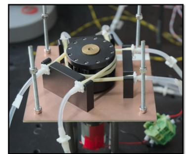
Fig. 3 – Peristaltic pump with phase-shifted tubings and head with 12 rolls.
