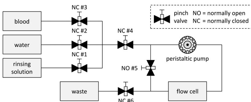
Fig. 1 – Schematic diagram of the constructed fluidic circuit. It allows a remote controlled automation of several processes, e.g. sample insertion, circulation or cleaning the circuit.
