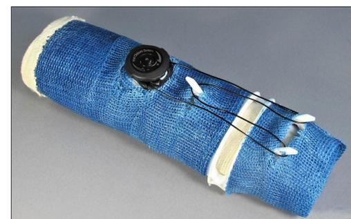
Fig. 5- Assembled prototype of cast system. The forearm phantom is covered with a cotton cast sleeve and the redesigned cast attachment (3D-printed from polyamide 12) is placed over the sleeve. Synthetic casting material secures the cast attachment to the forearm.
