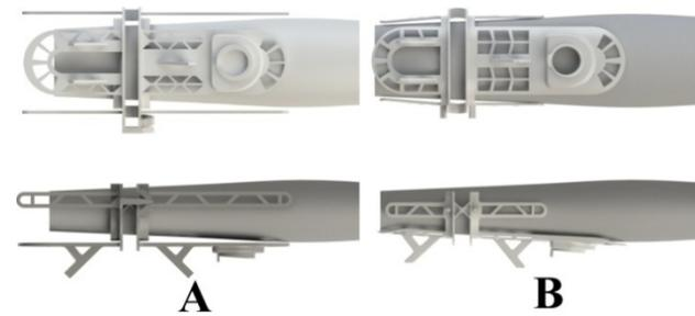
**Figure 5:** (A) original and (B) redesigned cast attachment. New design accommodates pediatric forearm dimensions, reducing gaps between padding and cast attachment components.
