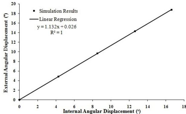
**Figure 4:** External versus internal angular displacement. Markers indicate calculated simulation values with a corresponding linear regression and an  $R^2$  value of 1.
