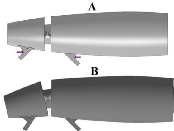
**Figure 2:** Mechanical behavior of total cast system (A) before and (B) after the external load is applied. An external closure mechanism applies a horizontal force (purple vectors) at each hook, creating a hinge-like reaction at the truss joint.
