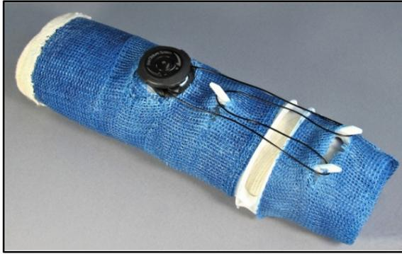
**Figure 6:** Final assembled prototype of redesigned cast system.
