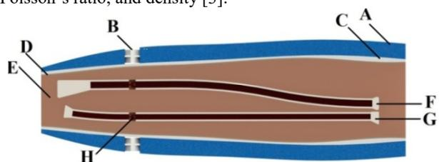
**Figure 3:** Cross-section of CAD forearm model and cast system: (A) casting material, (B) imbedded cast attachment, (C) padding, (D) skin, (E) soft tissue, (F) radius, (G) ulna, (H) fracture site (modeled as hinge joint).
