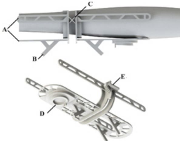
**Figure 1:** The cast attachment is positioned on the patient's arm after padding is in place: (A) main body, (B) guide hooks, (C) truss joint, (D) dial mount, (E) corrective angle indicator.
